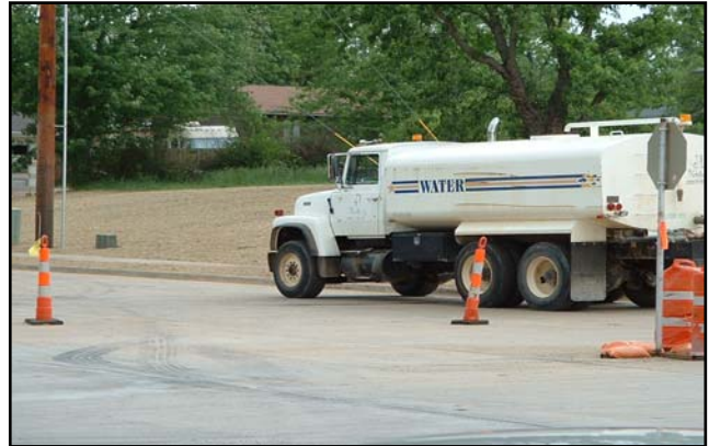
Water truck used for dust control
