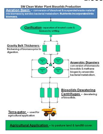
The Southwest Plant generates approximately 16 dry tons of biosolids per day. The biosolids are processed and utilized as a soil conditioner and fertilizer. Biosolids hauled from the Northwest Clean Water Plant are also processed at the Southwest Plant. See the biosolids page for more information.
